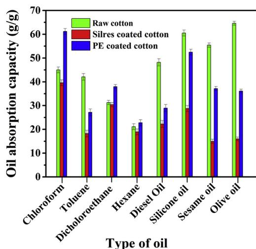
Fig. 8. The absorption capacities (weight gains) of bare, SCC and PE-CC fibers for different oils and organic solvents.
