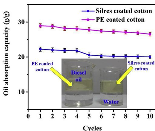
Fig. 12. The change of oil absorption capacity of the SCC and PE-CC fibers as a function of the number of recycling is plotted. Photographs of SCC and PE-CC fibers after more than 10 recycling process were stably floated on water surface even after 3 days are shown in the inset.
