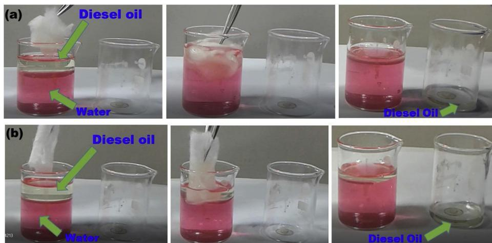
Fig. 7. Separation of diesel oil from water surface using (a) SCC and (b) PE-CC as absorbent.
