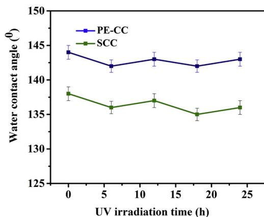
Fig. 11. Effect of UV-irradiation time on water contact angle of the prepared PE-CC and SCC fibers.
