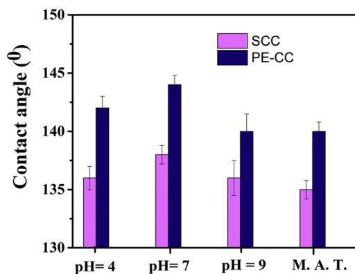
Fig. 9. The water contact angle of hydrophobic SCC and PE-CC after immersion in solutions at different pH (4, 7 and 9) values for 12 h and after mechanical abrasion test (M.A.T.).
