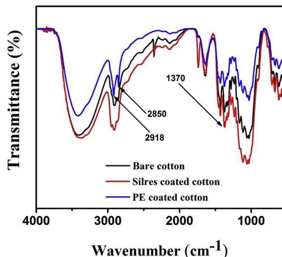
Fig. 5. FTIR spectra of the bare, silres coated and PE coated cotton fibers.
