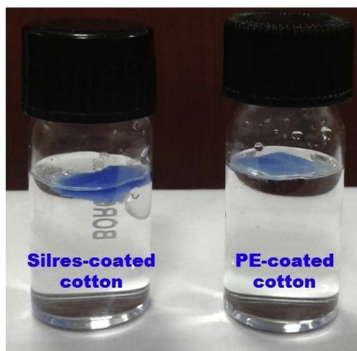
Fig. 10. Oil wetted SCC and PE-CC were placed on the surface of clean water. After 24 h, the oil wetted samples were not dipped in water, showing stability of coatings.
