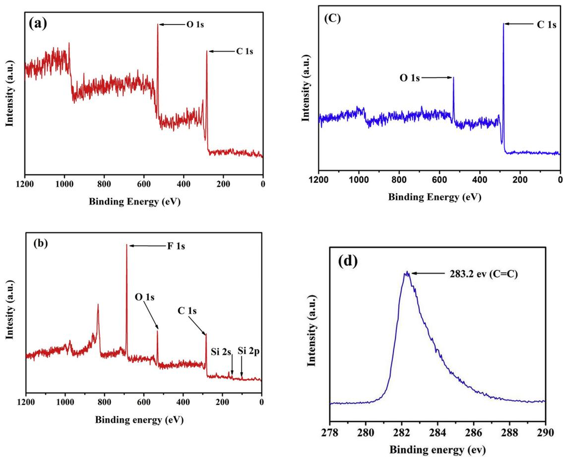
Fig. 6. XPS spectra of (a) uncoated cotton fibers (b) SCC and (c) PE-CC fibers (d) high resolution of C 1s peak in PE-CC.
