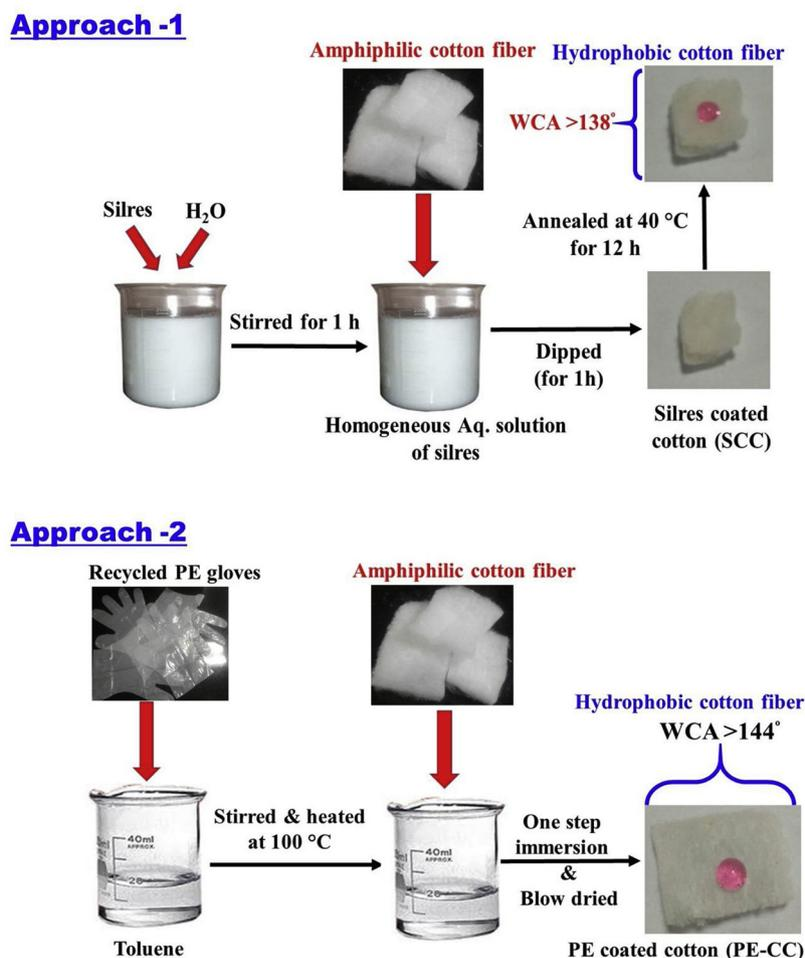
Fig. 1. Schematic illustration of procedure for the fabrication of hydrophobic fibers SCC (approach-1) and PE-CC (approach-2) via dissolution and immersion approach.
