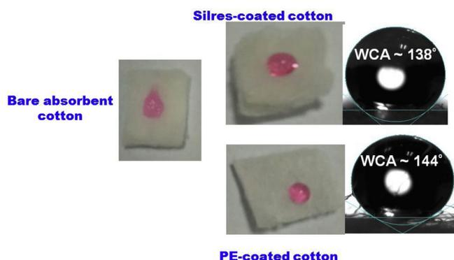
Fig. 2. Optical Images of water droplets (dyed with phenosafranin) on the bare, silres coated and PE-coated cotton surface with the water contact angle.
