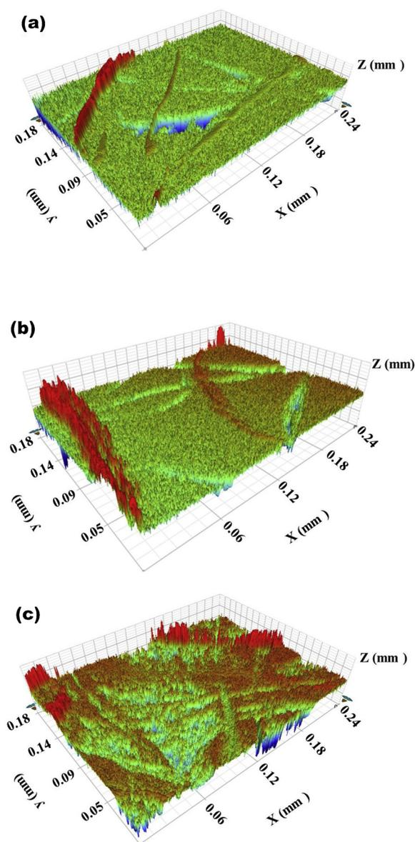
Fig. 4. Optical profiler images of the surface of (a) raw cotton (b) SCC and (c) PE-CC fibers.
