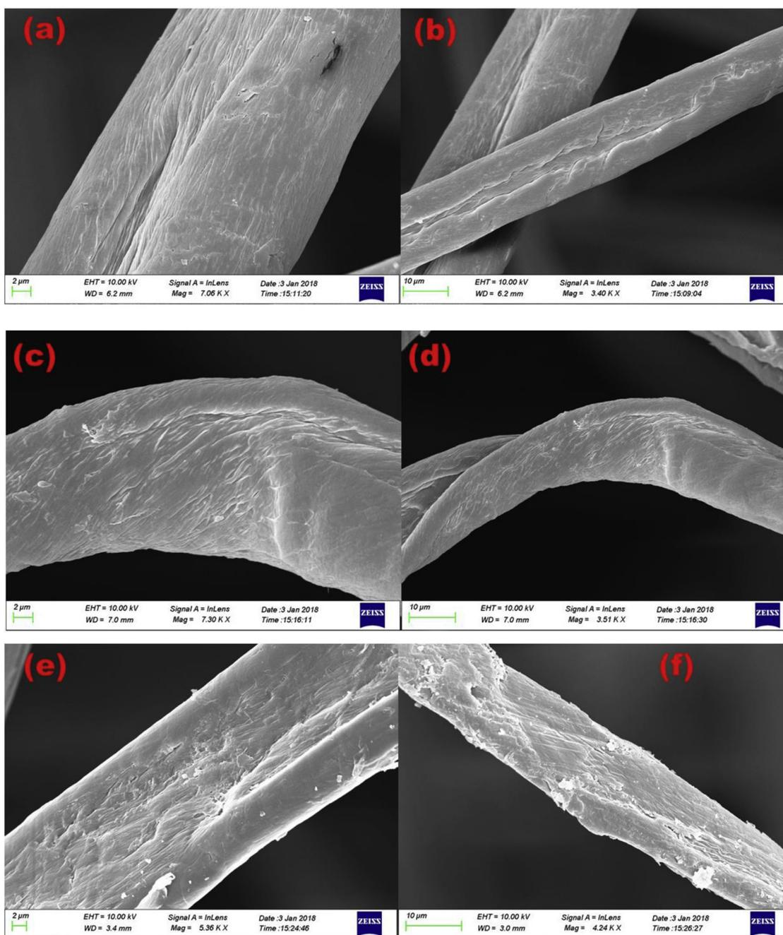
Fig. 3. SEM images of raw cotton (a) low and (b) high magnification, SEM images of SCC in (c) low and (d) high magnification and SEM images of PE-CC in (e) low and (f) high magnifications.
