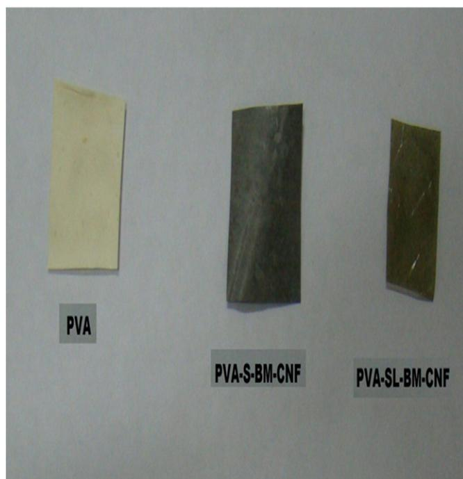
Fig. 8. Photographs of prepared PVA-M, PVA-S-BM-CNF, and PVA-SL-BM-CNF films.
