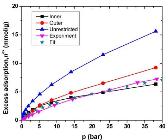
**Figure 4.** Excess adsorption amount of CO<sub>2</sub> in double-walled carbon nanotube arrays with  $r = 2.5$  nm and  $d = 15$  nm, for different modes of adsorption.  $T = 303$  K.
