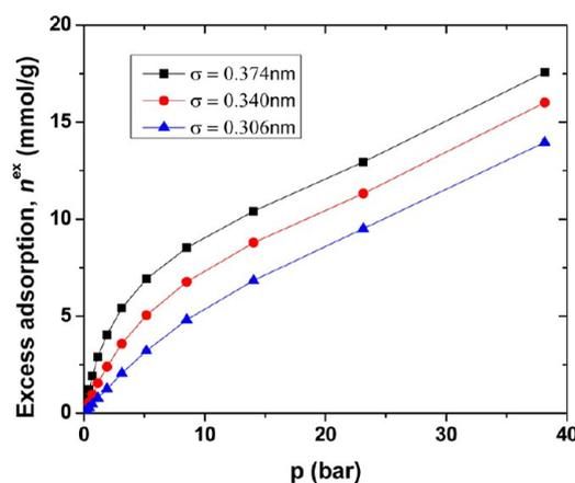
**Figure 13.** Excess adsorption amount of CO<sub>2</sub> in double-walled carbon nanotube arrays with  $r = 2.5$  nm and  $d = 2$  nm for unrestricted adsorption and different values of the Lennard-Jones energy parameter  $\sigma$  of the CNT carbon,  $T = 303$  K.
