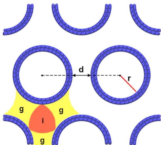
**Figure 1.** Schematic arrangement of double walled CNTs as used in this work, with internal radius  $r$  and intertube (surface-to-surface) distance  $d$ . Interstitial and groove regions are represented by symbol  $i$  and  $g$ , respectively.
