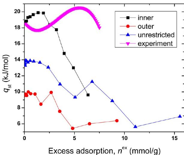
**Figure 6.** Isotheric heat of adsorption for different modes of adsorption of CO<sub>2</sub> in double-walled carbon nanotube arrays with  $r = 5.0$  nm and  $d = 15$  nm at  $T = 303$  K.
