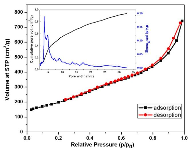
**Figure 3.** Nitrogen adsorption–desorption isotherm at 77 K for the as-prepared 3D aligned CNT sample,  $p_0 = 1$  bar. The inset shows the pore size distribution using nonlinear density function theory<sup>25,26</sup> as measured using the Quantachrome Autosorb.
