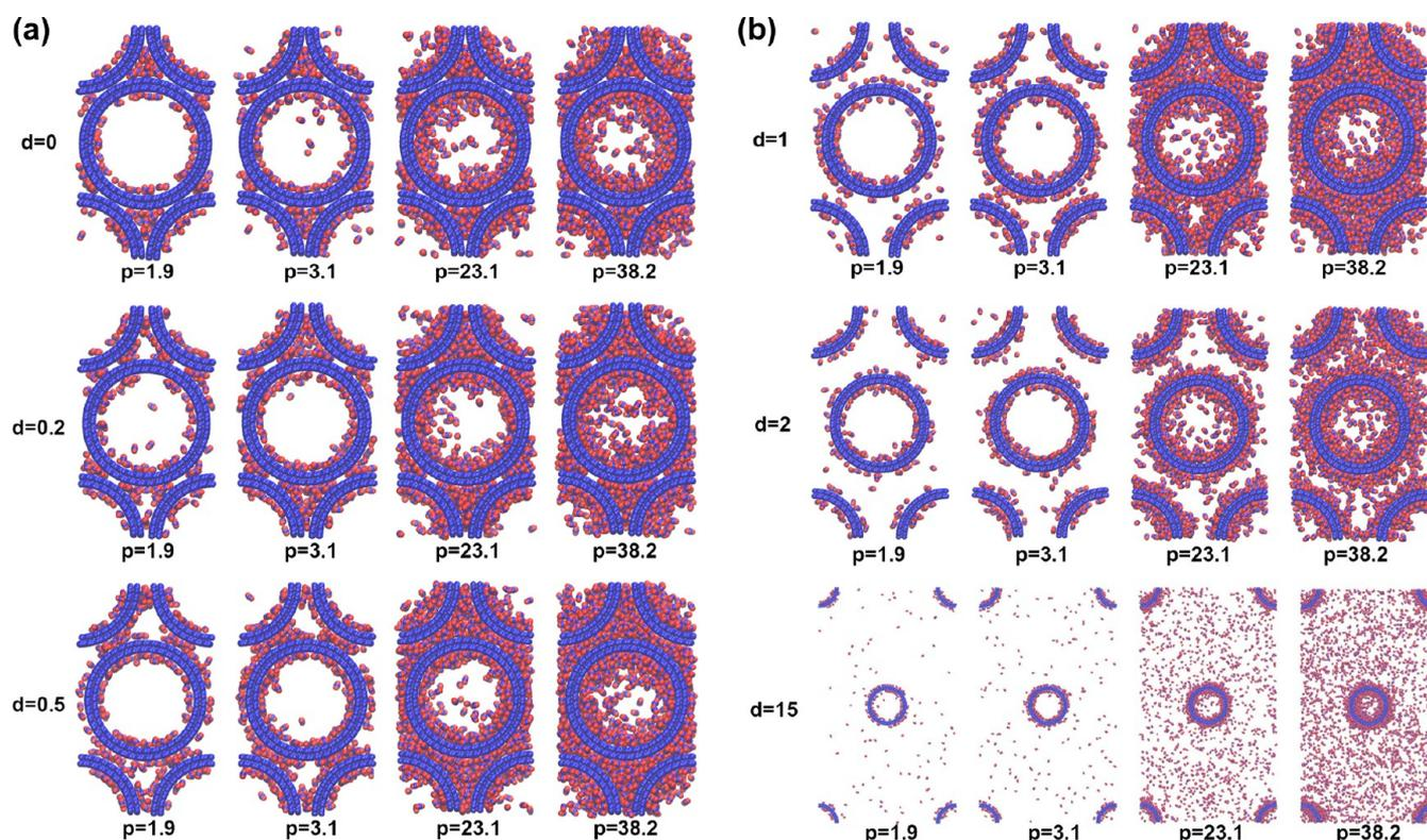
**Figure 9.** Snapshots of carbon-dioxide molecules in double-walled carbon nanotube arrays for unrestricted adsorption: (a) rows from top to bottom:  $d$  (nm) = 0, 0.2, and 0.5 (b): rows from top to bottom:  $d$  (nm) = 1, 2, and 15. Columns from left to right correspond to  $p$  (bar) = 1.9, 3.1, 23.1, and 38.2.
