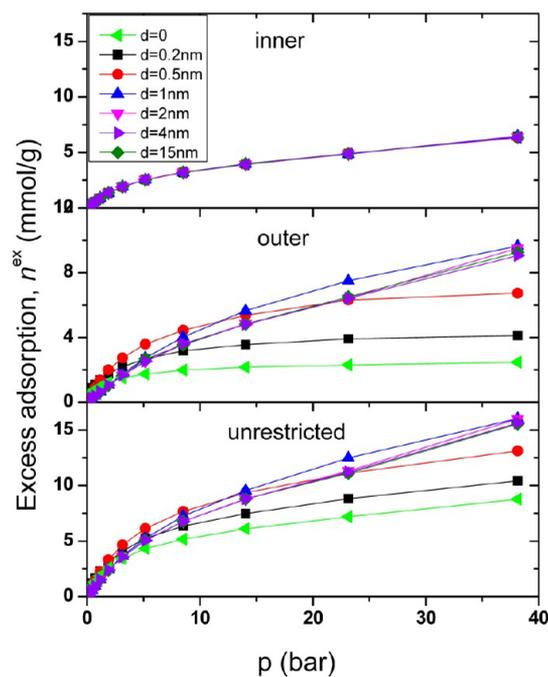
**Figure 8.** Excess adsorption isotherm of CO<sub>2</sub> in double-walled carbon nanotube arrays with radius,  $r = 2.5$  nm. Intertube distance,  $d$ , is varied from 0 to 15 nm.
