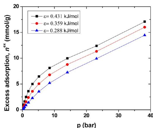
**Figure 12.** Excess adsorption amount of CO<sub>2</sub> in double-walled carbon nanotube arrays with  $r = 2.5$  nm and  $d = 2$  nm for unrestricted adsorption and different values of the Lennard-Jones energy parameter  $\epsilon$  of the CNT carbon,  $T = 303$  K.
