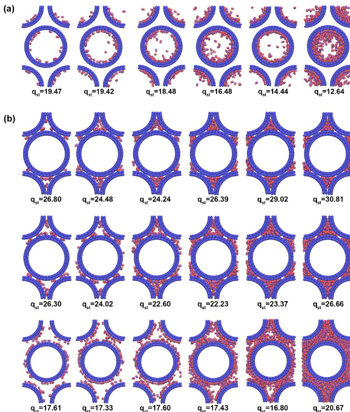
**Figure 11.** Snapshots of carbon-dioxide molecules in double-walled carbon nanotube arrays for adsorption modes at different  $q_{st}$  values. (a) Inner adsorption,  $d = 0.5$  nm. (b) Outer adsorption, rows from top to bottom correspond to  $d = 0.0, 0.2,$  and  $1.0$  nm.  $q_{st}$  values are displayed at the bottom of the snapshots.
