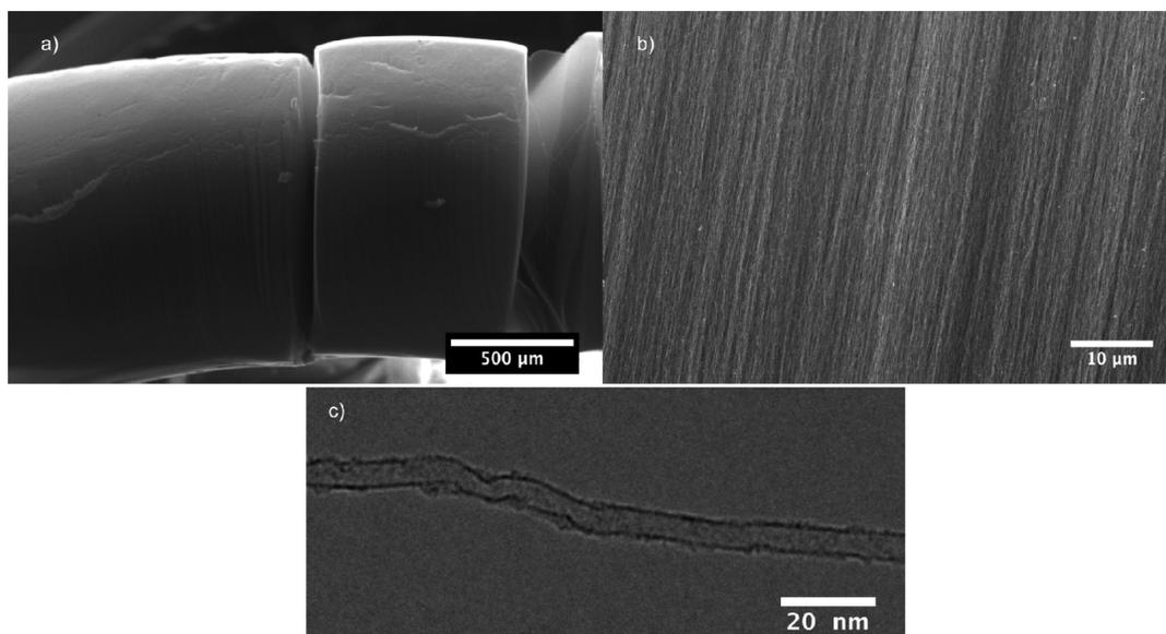
**Figure 2.** (a) SEM image of 3D aligned CNT block structure, (b) magnified image demonstrating the vertical alignment of the CNTs within such an array, and (c) TEM image of an individual double walled CNT ( $\sim 5$  nm inner diameter) unhinged from a CNT block by ultrasonification.
