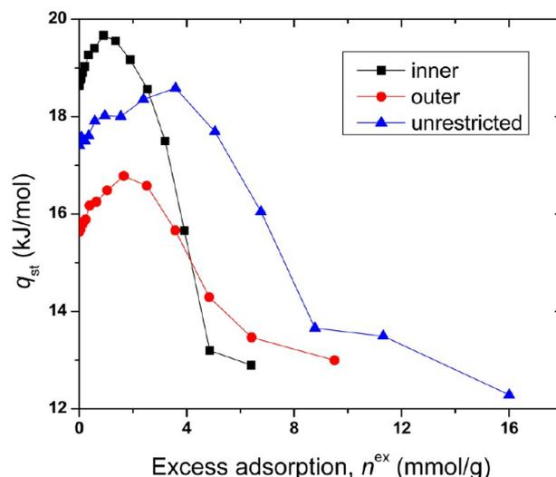
**Figure 7.** Isotheric heat of adsorption for different modes of adsorption of CO<sub>2</sub> in double-walled carbon nanotube arrays with  $r = 2.5$  nm and  $d = 2$  nm at  $T = 303$  K.
