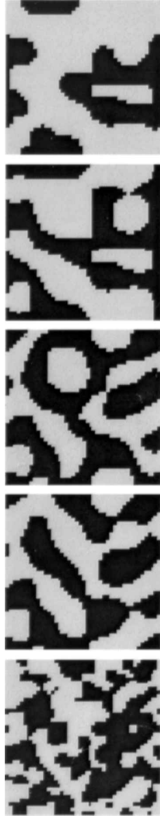
Figure 12. Two-color representation of the film morphology in a 25 nm thick film. Black and gray represent the regions above and below the mean thickness, respectively. The images correspond to (from left to right) I_N (\times 10^{-9}) = 1.6, 100, 180, 280, and 600 nm, respectively. I_N is as defined in Fig. 10.
